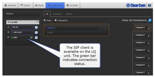
5. Go to the **Assignments** page of the CCM. Bring both the External port and the SIP port together in a **Channel**.
