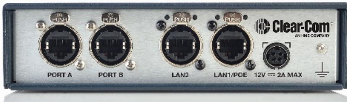
Two 4-wire connectors (etherCON RJ45)
