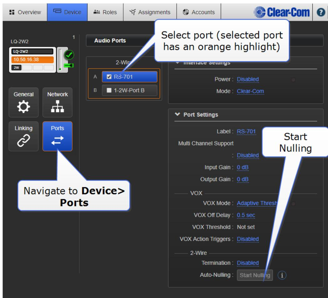
**Note:** The auto-nulling operation emits a loud hiss on the circuit. When auto-nulling, ensure that all talk buttons on external Partyline devices are turned off.
